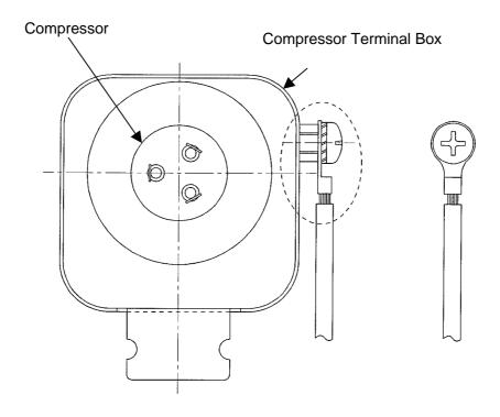
Earthing Terminal ( Delivery under the M6 bolt and Terminal box is installed )
